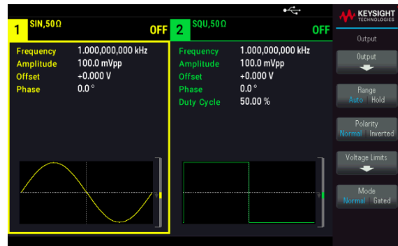
Figure 2. Dual-screen display of standard sine and square wave
