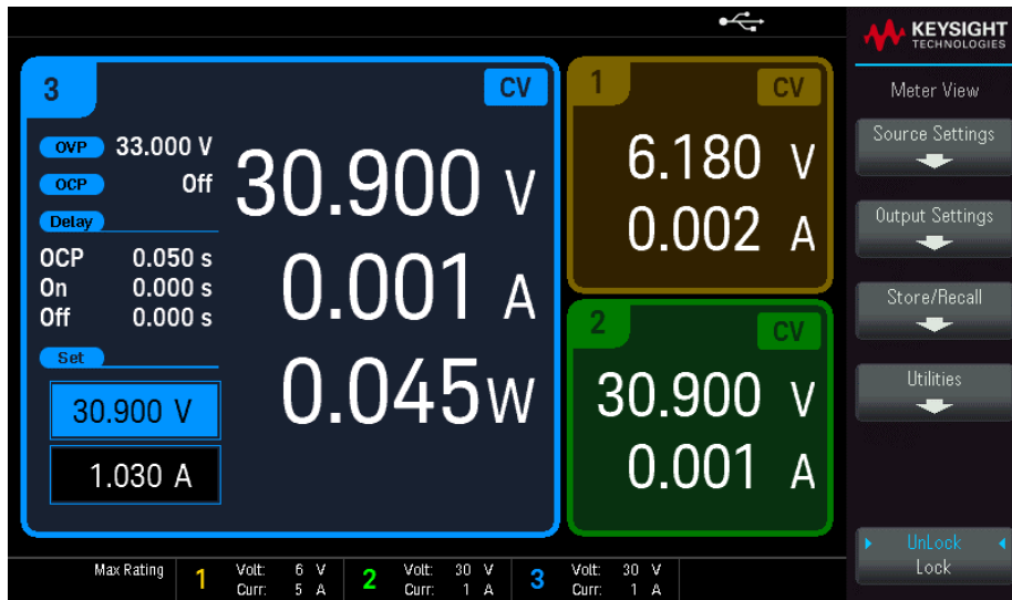
Figure 2. View details of a single channel including the measured power, OVP/OCP condition, and delays.
