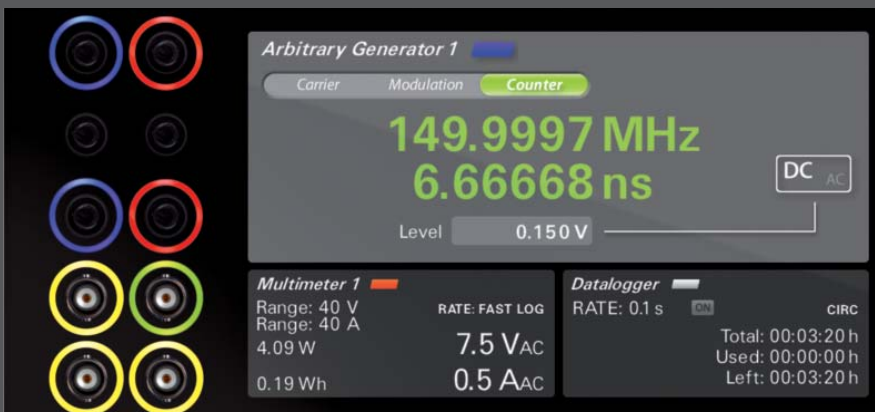
Integrated counter: Allows the acquisition of AC and DC signals as well as the adjustment of the trigger level in the DC area which is as standard up to 150 MHz. Optional increase of the measuring range to 1,5 GHz (Ref. No. EL5.F1G)
