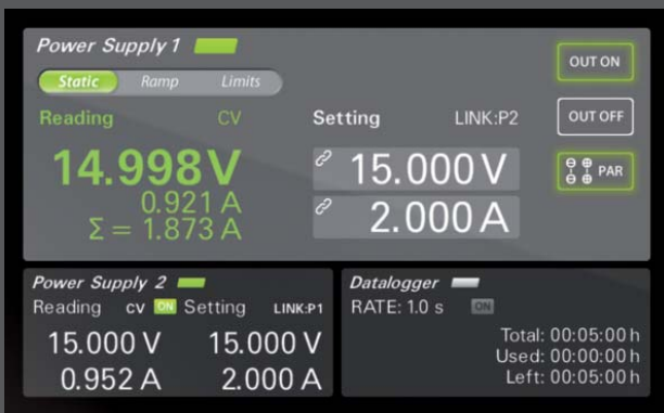
Optional comfort equipment (Ref. No. EL5.C): Internal serial/parallel connections of power control units with residual current indication.
