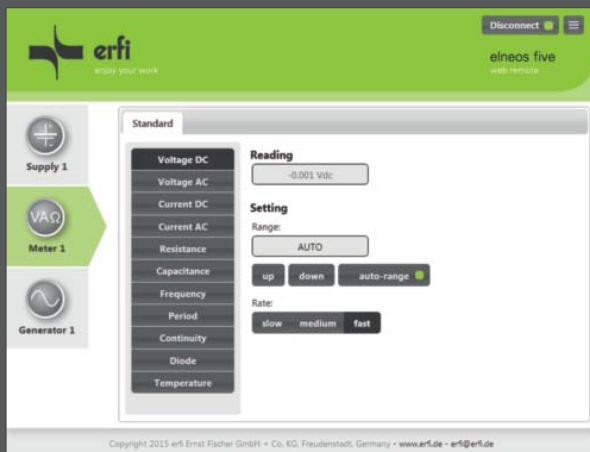
Telecontrol digital multimeter: The web server allows the complete telecontrol and the display of measured values of all functions.
