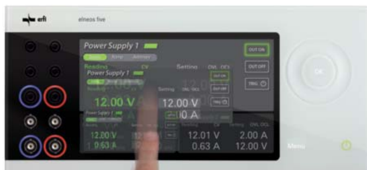
Changing the devices from the secondary to the primary area by 1-finger gesture.
