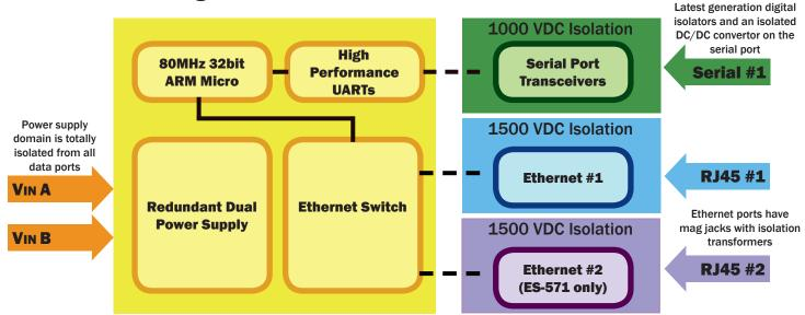
This device has 4 galvanically isolated power domains each with a minimum of 1,000 VDC isolation, ensuring data communications and power lines are protected from damaging electromagnetic interference.
