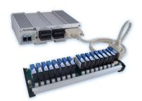
Interface to microBlox® uB signal conditioning modules.
