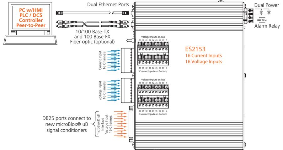
32 analog inputs (16 current + 16 voltages) ♦ Modbus TCP/IP, UDP/IP, i2o® peer-to-peer communication
