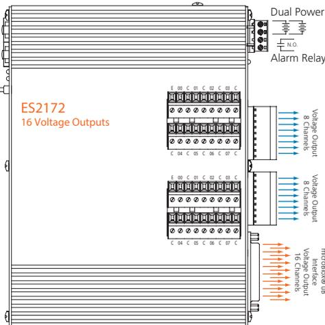
16 analog voltage outputs ♦ Modbus TCP/IP, UDP/IP, i2o® peer-to-peer communication
