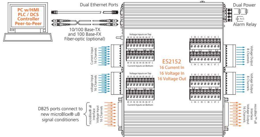
32 analog current/voltage inputs ◆ 16 analog voltage outputs ◆ Modbus TCP/UDP, i2o communication
