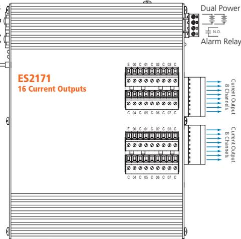
16 analog current outputs ♦ Modbus TCP/IP, UDP/IP, i2o® peer-to-peer communication
