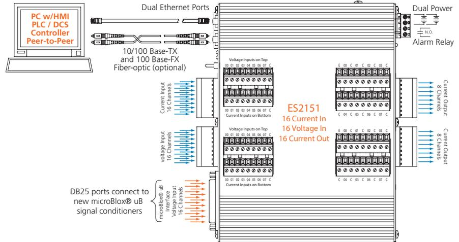
32 analog current/voltage inputs ◆ 16 analog current outputs ◆ Modbus TCP/UDP, i2o communication
