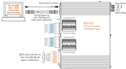
32 analog inputs (16 current + 16 voltages) ◆ Modbus TCP/IP, UDP/IP, i2o® peer-to-peer communication
