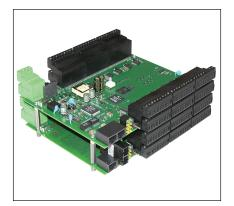
ESA-OMK open board stacking kit. One kit supplies standoffs to stack two units.
