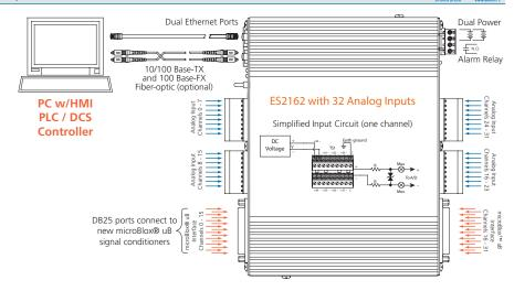
32-channel differential analog voltage input with uB interface
