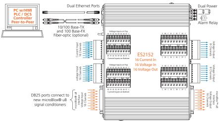
32 analog current/voltage inputs ◆ 16 analog voltage outputs ◆ Modbus TCP/UDP, i2o communication
