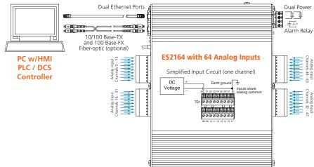
64-channel single-ended analog voltage input ◆ Modbus TCP/IP or UDP/IP communication
