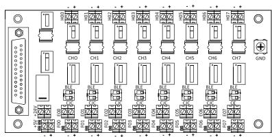
High-density isolation amplifiers ◆ Parallel interface connects to Ethernet Analog Input Modules
