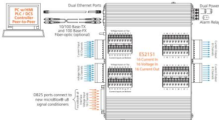
32 analog current/voltage inputs ◆ 16 analog current outputs ◆ Modbus TCP/UDP, i2o communication
