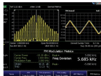
Characterize AM/FM signals using AM/FM demodulation
