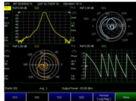
Simultaneously measure and view all four S-parameters, with a single connection
