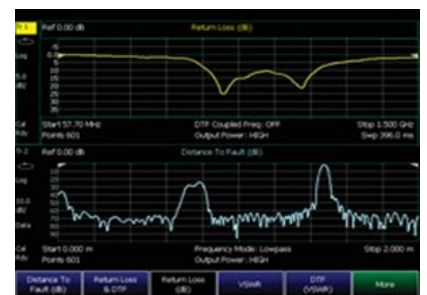
View return loss and DTF simultaneously
