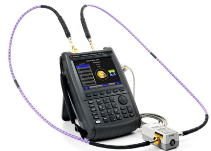
Perform fast and accurate calibrations using ECal
