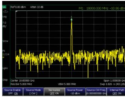
Use the internal microwave signal source for transponder testing
