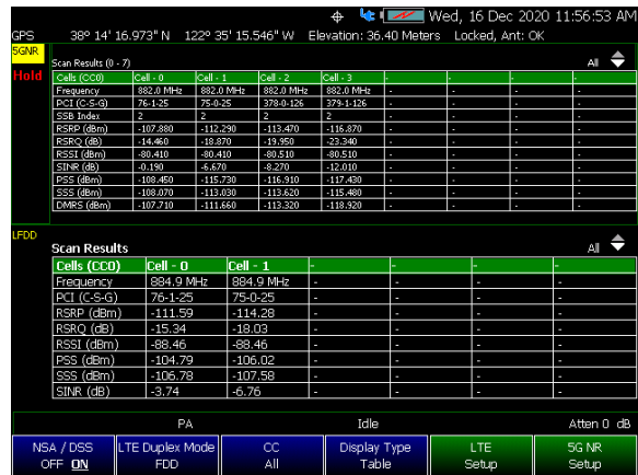
5G DSS on LTE channel Top: 5G NR channel scan with cell ID Bottom: LTE channel scan with cell ID
