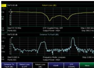
View return loss and DTF simultaneously
