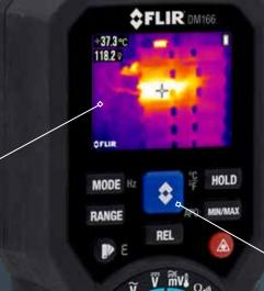
80 x 60 thermal imager to quickly scan for overheating components
