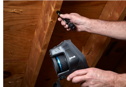
Use MR40 to confirm whether the cold spot found in a thermal image is moisture
