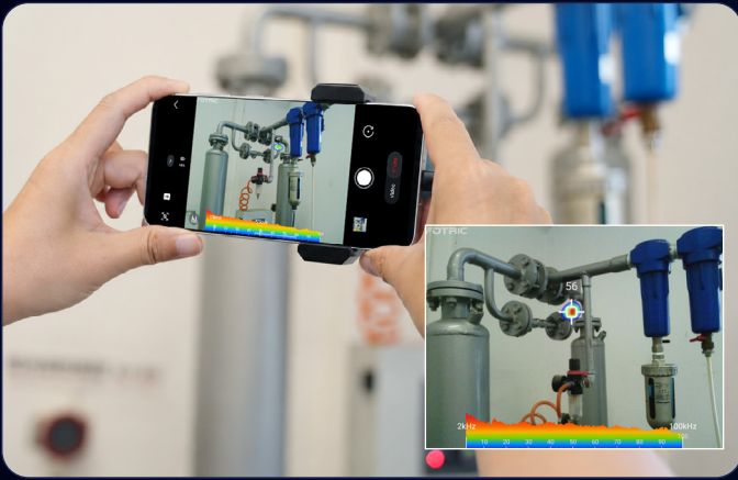
Compressed Air Leak/Vacuum Leak Inspection
