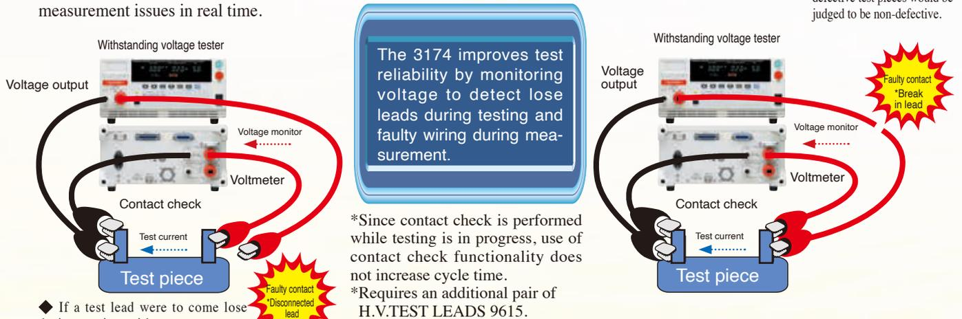
◆ If a test lead were to come loose during testing with a measurement device that does not offer contact check functionality, defective test pieces would be judged to be non-defective.
