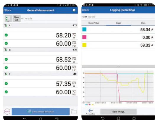
Review + + measurement data on a tablet with the distribution panel closed. You can also collect and review data measured at multiple locations, for example A, B, and C in the figure above. The app also provides simple logging functionality.
