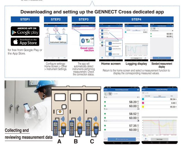
Review + + measurement data on a tablet with the distribution panel closed. You can also collect and review data measured at multiple locations, for example A, B, and C in the figure above. The app also provides simple logging functionality.
