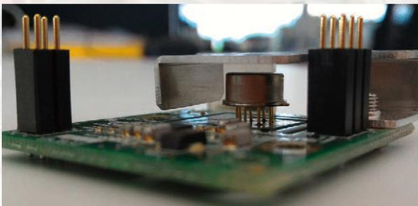
The voltage reference in the core represents screened components that have passed our special in-house tests and undergone long-term evaluation before being embedded in the system. Combining this with HIOKI's original fully automatic "Self-calibration" technology, we are able to offer a 1-year guaranteed 9ppm accuracy (DM7276).
