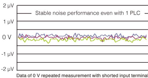
Circuit designs which minimize the effect temperature changes have on sensitive receiving components and Self-Calibration provide stable measurement.
