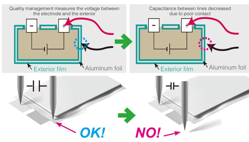
External potential measurement is effective for detecting poor insulation in the external film of lithium-ion batteries. For measuring devices such as a lithium-ion battery with a molded exterior, not only accuracy but probe contact reliability is vital.
