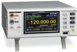
9 ppm voltage measurement accuracy
