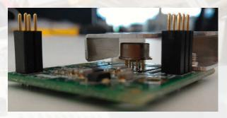
The voltage reference in the core represents screened components that have passed our special in-house tests and undergone long-term evaluation before being embedded in the system. Combining this with HIOKI's original fully automatic "Self-calibration" technology, we are able to offer a 1-year guaranteed 9ppm accuracy (DM7276).
