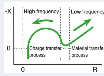
Measurement at low frequencies is necessary in order to measure characteristics such as ion behavior, and the IM3590 can conduct measurements at 1 mHz. The instrument's upper limit frequency is 200 kHz, allowing it to measure solution resistance.
