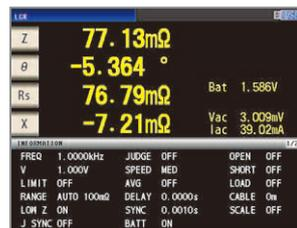
Measurement of alkaline batteries
