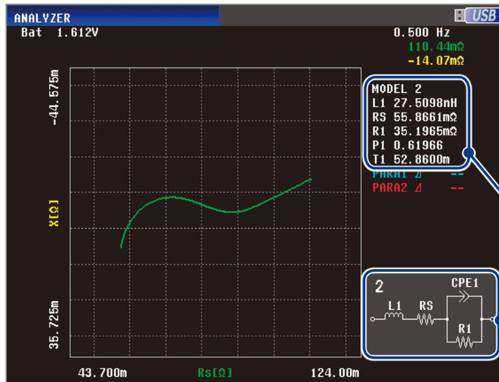
The ability to measure electrochemical components and materials makes possible evaluation by estimating equivalent circuits, facilitating a deeper understanding of reaction, electrode, and electrolyte characteristics. The IM3590 provides electrochemical component and material equivalent circuit models, allowing evaluation of solution resistance, charge transfer resistance, and electric double-layer capacitance.
