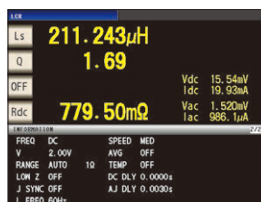
L, Q and Rdc continuous measurement screen
