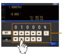
The judgment standard is calculated based on the measurement range and judgment reference value (valid setting range: 0% to 30,000%).
