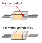
The contact check function measures the contact resistance between  $L_{\text{POT}}$  and  $L_{\text{CUR}}$  and between  $H_{\text{POT}}$  and  $H_{\text{CUR}}$  and displays an error if the readings are greater than or equal to a preset threshold.
