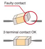
The Hi-Z reject function outputs an error if the measurement result exceeds a preset judgment standard. This capability enables the instrument to detect poor contact when performing measurement using a two-terminal fixture.
