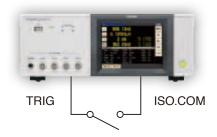
Select [External trigger] as the trigger setting and then control instrument operations such as measurement and saving of data from an external device such as a foot switch via the EXT. I/O terminal's TRIG signal.
