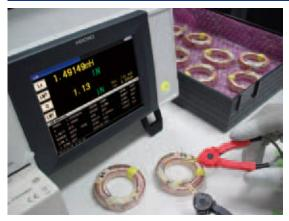
Save 32000 measurement results, copy them to a USB flash drive, and load them onto a computer. You can then open the measurement data using a spreadsheet to analyze variations and manage test data.
