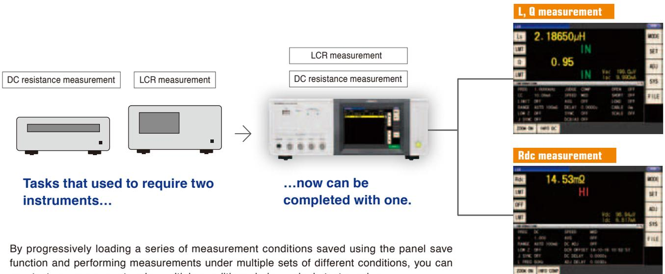
By progressively loading a series of measurement conditions saved using the panel save function and performing measurements under multiple sets of different conditions, you can now test one component under multiple conditions during a single test session.
