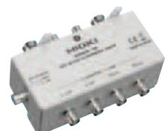
Measurement frequency range: 40 Hz to 2 MHz
