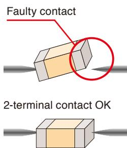
The Hi-Z reject function outputs an error if the measurement result exceeds a preset judgment standard. This capability enables the instrument to detect poor contact when performing measurement using a two-terminal fixture.
