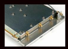
Each section uses a solid shield carved to match the on-board pattern or IC shape, thus reducing internal coupling. The shield
