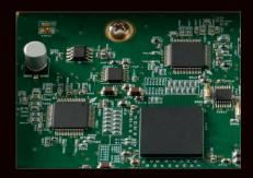
The measurement portion uses a high resolution A/D converter. By controlling the input signal's level and frequency, the A/D converter's dynamic range can be utilized to the fullest, achieving measurement with a wide impedance range and minimum variability.
