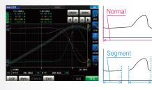
Perform measurement after setting the sweep parameter (frequency or level), sweep range, number of sweep points, and measurement conditions.
