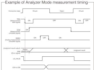
EOM: Off from trigger input to end of measurement processing INDEX: Off during probe chuck (probe cannot be removed from target)
