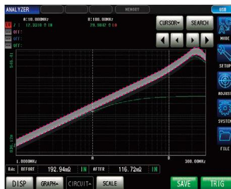
Set the judgment area and then check whether component measurement results fall inside that area. This approach is well suited to differentiating between defective and non-defective components.
