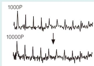
Scale by dB. Input the overall value (sum of the power spectrum) directly as a dB value.
