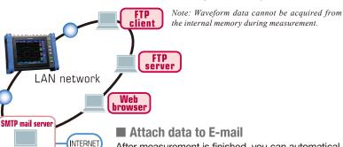
After measurement is finished, you can automatically send the captured data as an e-mail attachment. Data can also be transferred at you desired timing.
