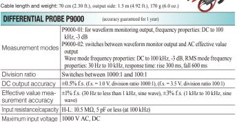
Maximum rated volt-1000 V AC, DC (CAT III) age to ground Operating -40°C to 80°C (-40°F to 176°F) temperature range (1) AC adapter Z1008 (100 to 240 V AC, 50/60 Hz), 6 VA (including AC adapter), 0.9 VA (main unit only) (2) USB bus power (5 V DC, USB-microB terminal), 0.8 VA Power supply (3) External power source 2.7 V to 15 V DC, 1 VA
