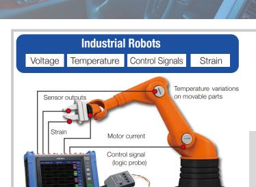
The plug-in module-based architecture means you can mix and record a variety of signals across multiple channels - ideal for verifying the operation of multi-axis robots.
