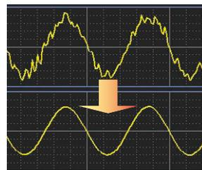
Results of a calculation-based simulation of a waveform from which high-frequency distortion has been rejected by passing it through a low-pass filter.
