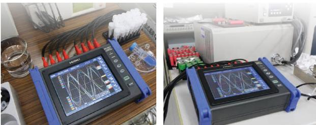
With its multi-channel, long-term recording capabilities, the **MR8875** is ideally suited for use in development applications such as performance and durability testing.
