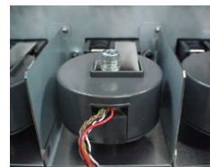
DCCT current sensor (in the PW3337)
