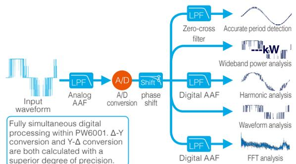
\* AAF (Anti-aliasing filter): This filter prevents aliasing errors during sampling.
