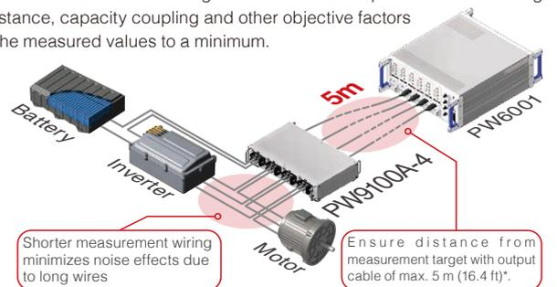
Shorter measurement wiring minimizes noise effects due to long wires
