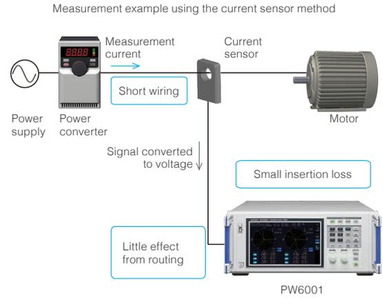
Compared to the direct wire connection method, measurement with conditions closer to the actual operation environment of a power converter is achieved.
