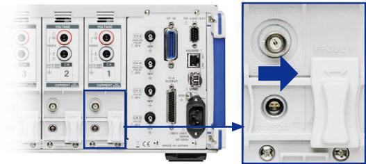
**Wideband probe terminal: Slide the cover to the right.**
