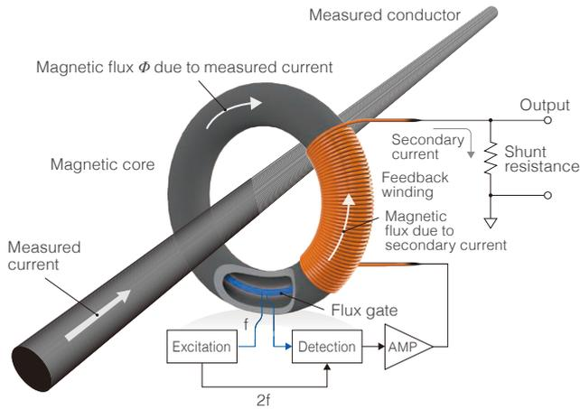
High-accuracy sensors use the "zero flux method (flux gate detection type)" as the measurement method. High-frequency currents are detected with the winding (CT method), and DC to low frequency currents are detected using a "flux gate."
