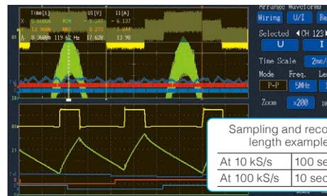
In addition to the level trigger function, the new event trigger starts recording when there is a fluctuation in RMS values or frequency. Cursor measurement and waveform zoom functions also render oscilloscopes unnecessary for waveform analysis.
