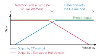
Wideband current sensors use the "zero flux method (Hall element detection type)" to measure. High-frequency currents are detected with the winding (CT method), and low frequency currents including DC are detected with the "Hall element."
