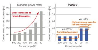
Combination of PW6001 and CT6904A Accuracy achieved when measuring the fullscale current in each range, 45 Hz to 65 Hz.
