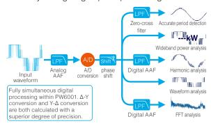
\* AAF (Anti-aliasing filter): This filter prevents aliasing errors during sampling.
