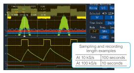
In addition to the level trigger function, the new event trigger starts recording when there is a fluctuation in RMS values or frequency. Cursor measurement and waveform zoom functions also render oscilloscopes unnecessary for waveform analysis.
