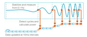
Even during frequency fluctuations from low to high, the fundamental waveform is automatically pursued. Comes equipped with  $\Delta$ -Y and Y- $\Delta$  conversion while calculating with a high degree of accuracy.
