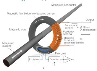
High-accuracy sensors use the "zero flux method (flux gate detection type)" as the measurement method. High-frequency currents are detected with the winding (CT method), and DC to low frequency currents are detected using a "flux gate."
