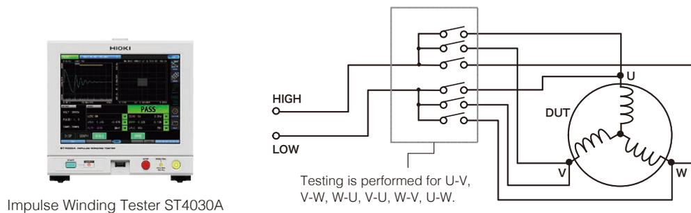
Automate testing using a setup such as the one shown below by using a High Voltage Scanner 3930 to switch the measurement circuit.
