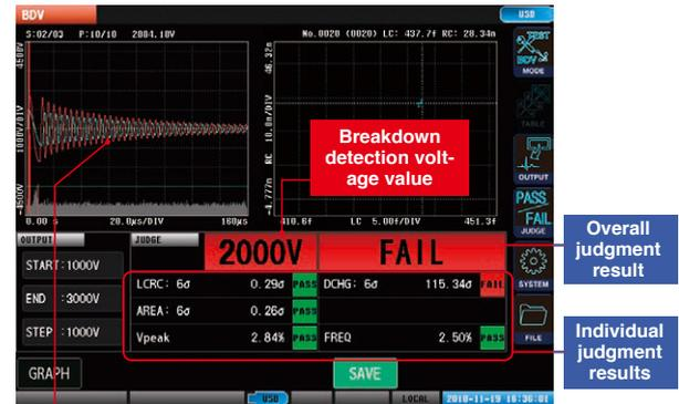
If any of the judgments yields a FAIL result, the insulation is considered to have started to break down, and testing is halted at that point. The breakdown voltage waveform is shown in red.
