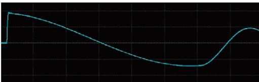
The captured waveform length is inadequate due to the response waveform's low oscillation frequency. The sampling frequency needs to be decreased.
