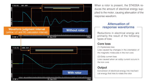
As long as the response waveforms for defective and non-defective motors differ, even if they are attenuated, the motors can be tested.
