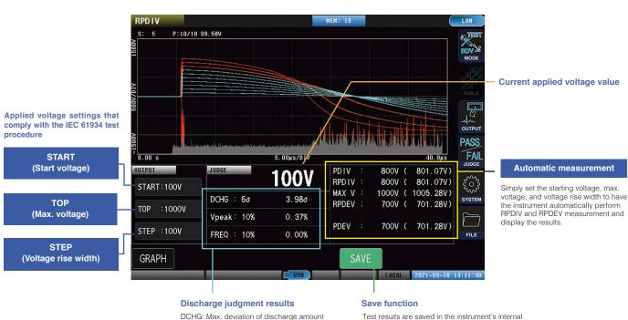
Vpeak: Max. deviation of discharge amount Vpeak: Max. misalignment width from the standard peak voltage value
