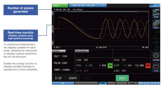
During continuous measurement, only measurement data for the most recent pulse is maintained by the ST4030A.
