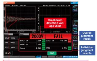
If any of the judgments yields a FAIL result, the insulation is considered to have started to break down, and testing is halted at that point. The breakdown voltage waveform is shown in red.
