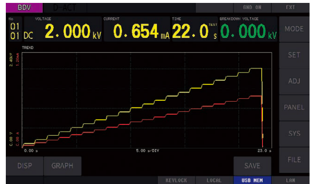
Example of stepped voltage rise testing
