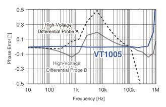
High-voltage differential probes have a broad frequency band, but measurement error on the order of several percent occurs within that band. Thanks to high accuracy and excellent frequency flatness within its frequency band, the VT1005 makes it possible to detect efficiency improvement effects on the order of 0.1%, a task that has been impossible until now.
