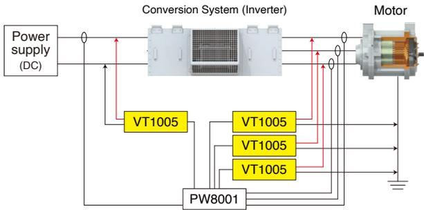
Evaluation of the Efficiency of Inverters that use SiC Power Devices in Electrical Railways
