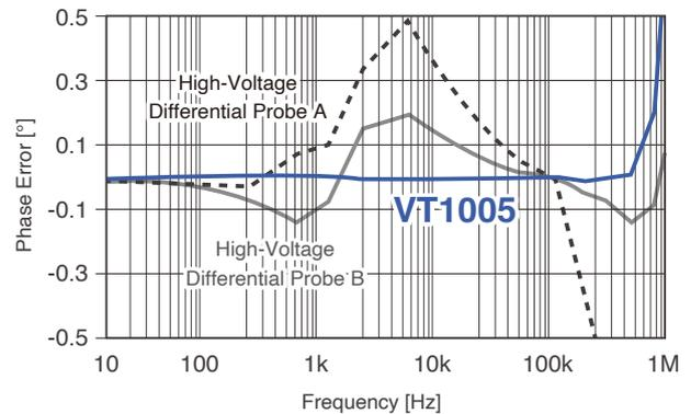
High-voltage differential probes have a broad frequency band, but measurement error on the order of several percent occurs within that band. Thanks to high accuracy and excellent frequency flatness within its frequency band, the VT1005 makes it possible to detect efficiency improvement effects on the order of 0.1%, a task that has been impossible until now.
