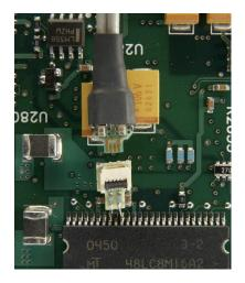
Figure 10: N5425B/26A differential ZIF head and ZIF tip
