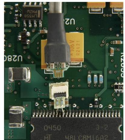
Figure 10: N5425B/26A differential ZIF head and ZIF tip
