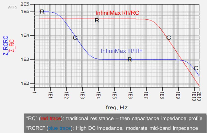
Figure 2: Input impedance vs frequency response plot of RC probes and RCRC probes
