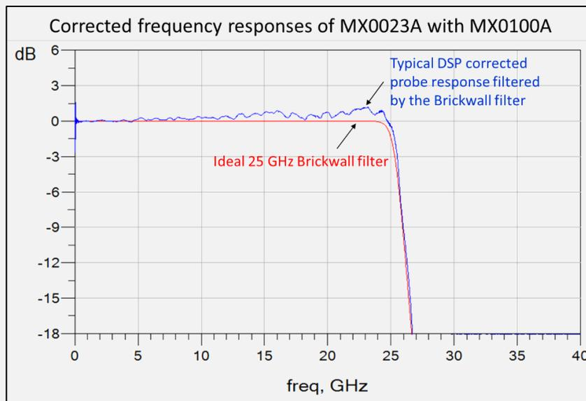
Figure 3: The unique s-parameters of the probe amp are used to flatten the magnitude and phase response of the probe for high accuracy measurements
