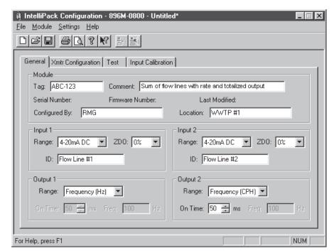
IntelliPack Configuration Software makes it very easy to set up your input and output ranges and other operational parameters.
