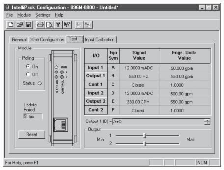
The test property sheet continuously displays polled information and input/output signal values for easy troubleshooting and diagnostic checkout.
