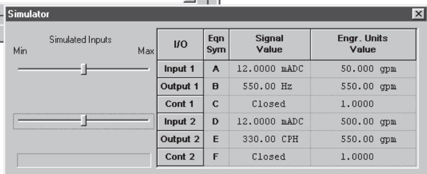
The pop-up simulator sheet helps you test equations in software with slider bars to simulate input conditions.
