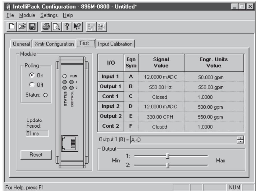
The test property sheet continuously displays polled information and input/output signal values for easy troubleshooting and diagnostic checkout.
