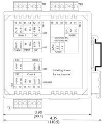
DC current input ◆ Single/dual-channel AC/DC-powered isolators ◆ Signal splitter
