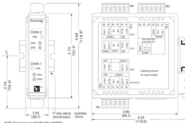
DC current input ♦ Single/dual-channel AC/DC-powered isolators ♦ Signal splitter
