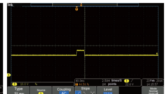
D/D Converter Surge Testing
