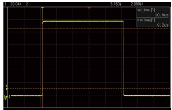
IT8733P+(150V, 120A, 600W) dynamic current curve(1A-120A), current slew 12A/us
