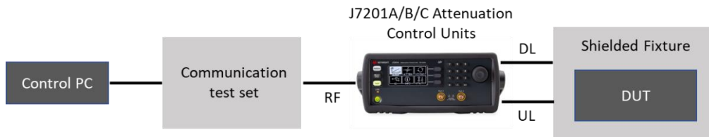
Figure 2. Simplified test setup for mobile receiver sensitivity test using a communication test set
