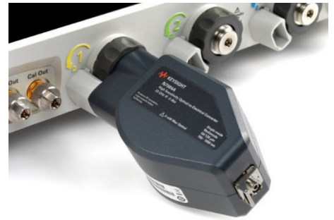
N7004A 33 GHz optical-to-electrical converter
