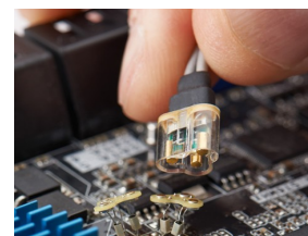
N2848A QuickTip head with N2849A QuickTip tips
