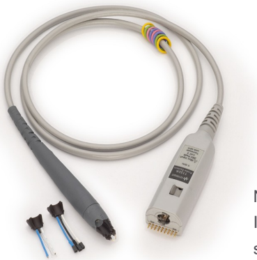
N2750A-02A InfiniiMode probe with standard accessories
