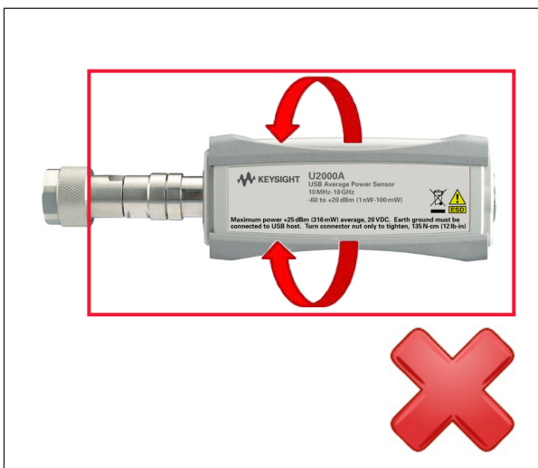
Figure 6. Do not turn the power sensor body
