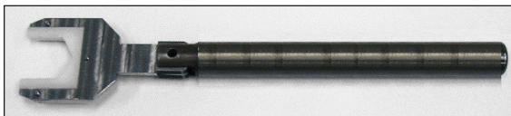
Figure 8. Straightened torque wrench
