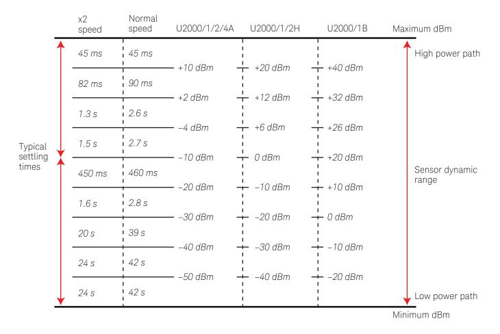
Settling time with auto filter, default resolution, and a 10 dB decreasing power step (not across the switching point) Settling time =  $25 \text{ ms}^{-1}$
