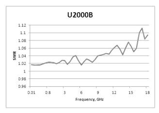
Typical SWR for U2000B sensor (25 °C ± 10 °C)
