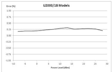
Typical power accuracy at 25 °C for U2000/1/2H sensors 1,2
