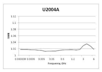
Typical SWR for U2004A sensor (25 °C ± 10 °C)
