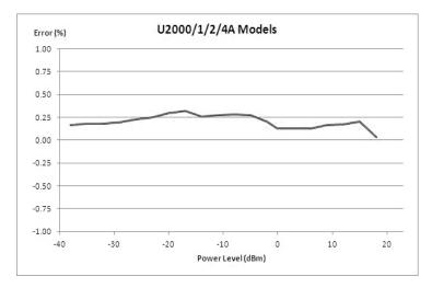
Typical power accuracy at 25 °C for U2000/1B sensors  $^{1,\,2}$
