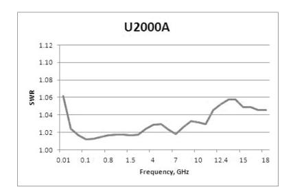
Typical SWR for U2001A sensor (25 °C  $\pm$  10 °C)
