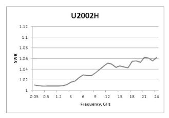
Typical SWR for U2002H sensor (25 °C ± 10 °C)
