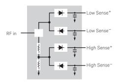
This technique ensures diodes in the selected signal path are kept in their square law region—with output current and voltage proportional to input power. The diode pair/attenuator/diode pair assembly can then yield the average of complex modulation formats across a wide dynamic range, irrespective of signal bandwidth.
