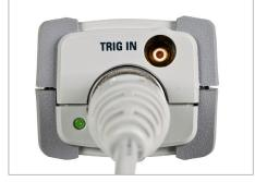
The external trigger input port on the U8481A.
