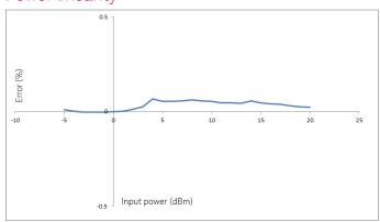
Figure 1. Typical U8480 Series power linearity at 25 °C with measurement uncertainty of  $\pm$  0.21%
