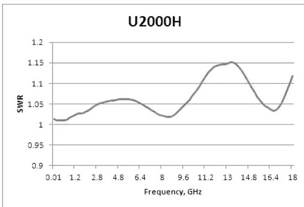
Typical SWR for U2000H sensor (25 °C ± 10 °C)
