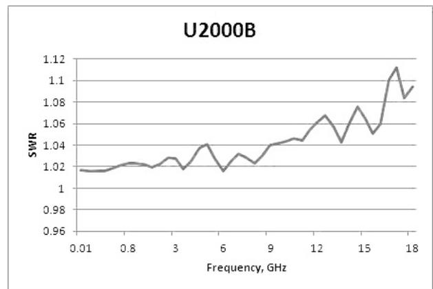
Typical SWR for U2000B sensor (25 °C ± 10 °C)
