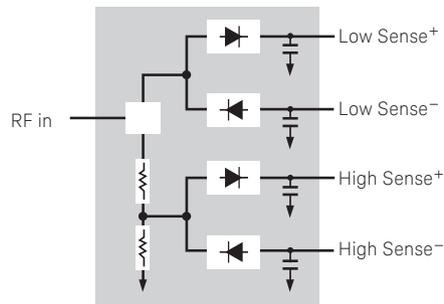
This technique ensures diodes in the selected signal path are kept in their square law region—with output current and voltage proportional to input power. The diode pair/attenuator/diode pair assembly can then yield the average of complex modulation formats across a wide dynamic range, irrespective of signal bandwidth.
