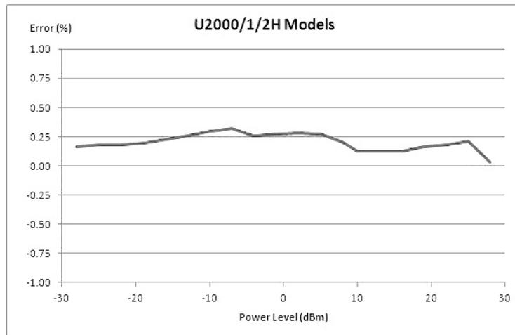
1. Measurement uncertainty  $\leq 1.9\%$ . At room temperature and excluding power level dependent terms (zero set, drift, and noise). Refer to Keysight Fundamentals of RF and Microwave Power Measurements (Part 3) Power Measurement Uncertainty per International Guide (Application Note 1449-3), 5988-9215EN for more information on measurement uncertainty.
