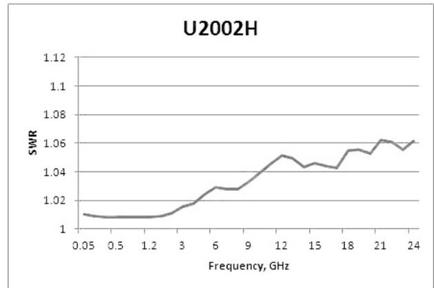
Typical SWR for U2002H sensor (25 °C ± 10 °C)
