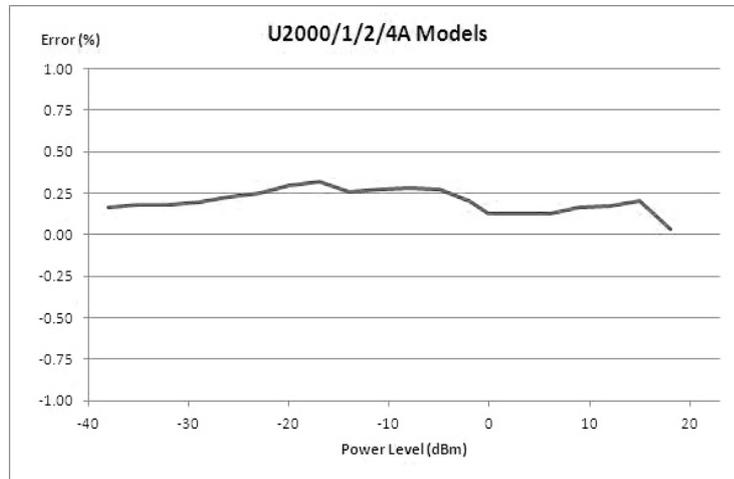
Typical power accuracy at 25 °C for U2000/1B sensors <sup>1, 2</sup>
