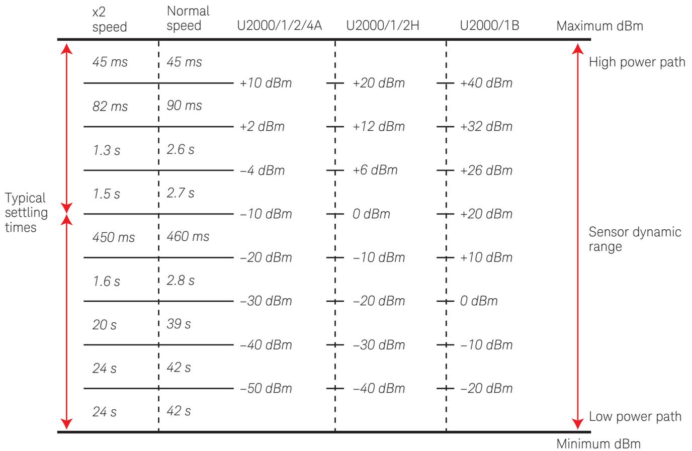
Settling time with auto filter, default resolution, and a 10 dB decreasing power step (not across the switching point)
