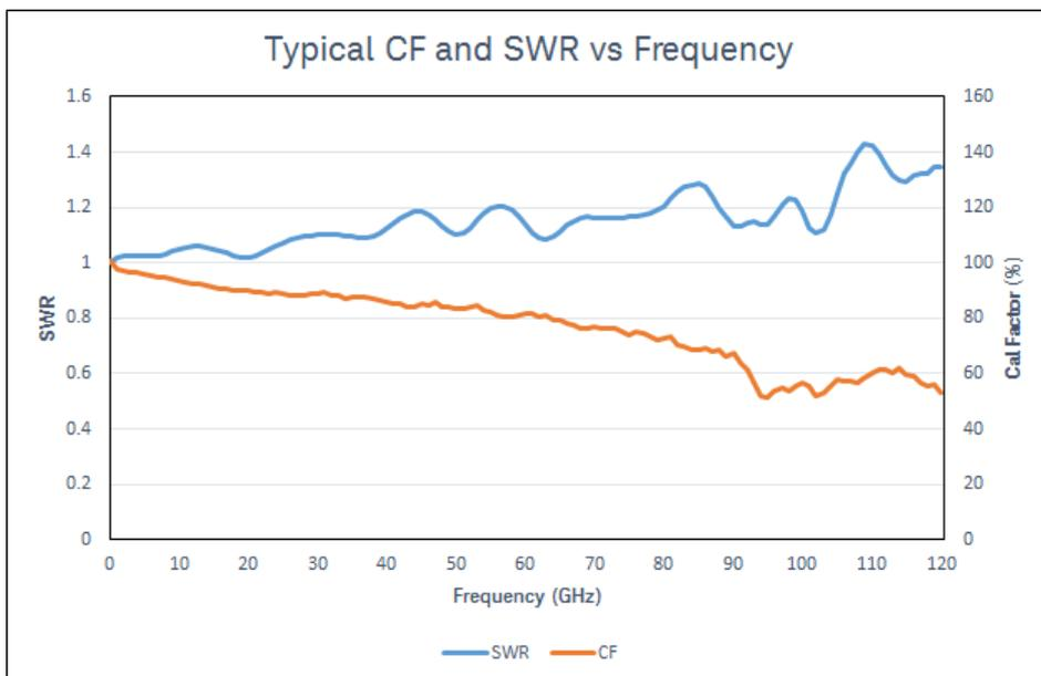
Figure 9. Typical calibration factor (CF) and SWR vs. frequency
